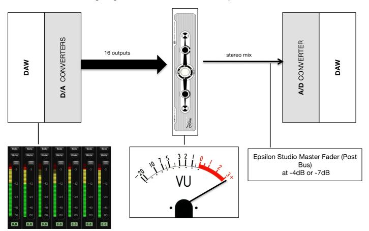
In a "saturated" mix the DAW output levels are "high". Inside our summing bus the signal levels are will be off the scale and the Epsilon Studio master fader requires attenuation. This is the same situation when using an analog console the master vumeters are off scale. The Epsilon Studio requires that the master fader attenuate the output levels to send the mix to DAW or other analog gear.
