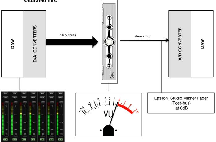
In a "clean" mix the DAW output levels are normal or "low". Inside our summing bus the signal levels are will be closet o 0VU=+4dBu and the Epsilon Studio master fader doesn't require attenuation, it's positionated at 0dB. **Remember:** the master fader is post-summing bus.
