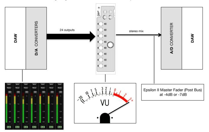
In a "saturated" mix the DAW output levels are "high". Inside our summing bus the signal levels are will be off the scale and the Epsilon II master fader requires attenuation. This is the same situation when using an analog console the master vumeters are off scale. The Epsilon II requires that the master fader attenuate the output levels to send the mix to DAW or other analog gear.
