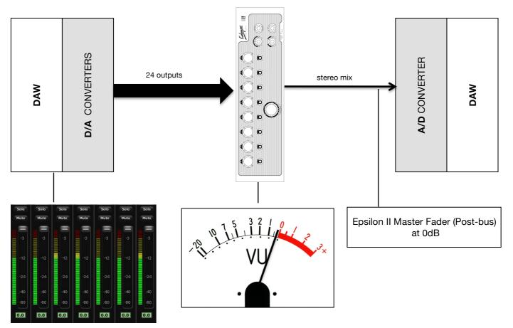
In a "clean" mix the DAW output levels are normal or "low". Inside our summing bus the signal levels are will be closet o 0VU=+4dBu and the Epsilon II master fader doesn't require attenuation, it's positionated at 0dB. **Remember:** the master fader is post-summing bus.
